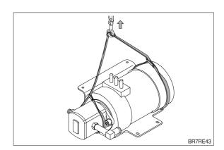
⑥ Remove 2 socket bolts fastening the pump & motor and then disengage the pump from motor.
