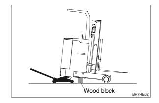
② Remove 6 flange bolts attaching the drive wheel and take off the drive wheel assembly.
