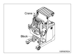
While supporting lift chains, remove the split pins and slide out chain anchor pins from the chain anchors of stationary upright.
