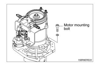
(10) Remove drive unit mounting bolts and pull out the drive unit by lifting with eyebolts on motor mounting tap. (M8 × 1.25)
