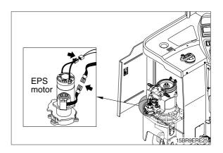
④ Loosen bolts and remove EPS motor assembly.
