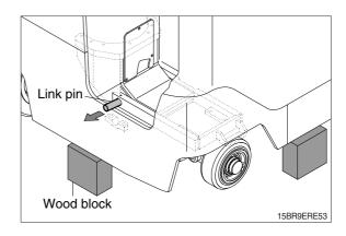
(5) Tire wire rope around the bracket and lift up slowly.
