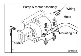
⑤ Tire wire rope around the hydraulic pump & pump motor assembly and lift up slowly.
